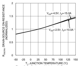
Figure 6. On-Resistance Variation with Temperature
