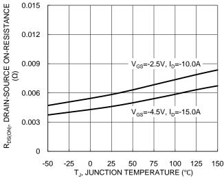
Figure 7. On-Resistance Variation with Temperature
