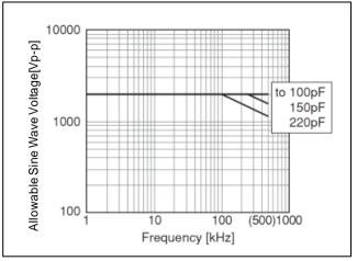
Frequency VS Allowable Sine Wave Voltage
