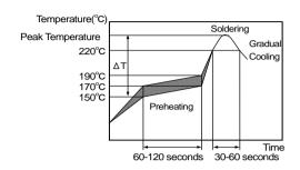
[Allowable Reflow Soldering Temperature and Time]
