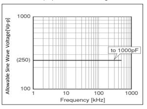
Frequency VS Allowable Sine Wave Voltage
