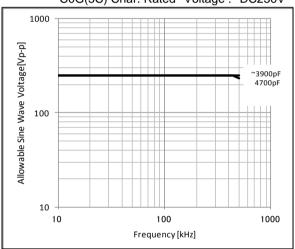
Except for 2012M/0805 and 3216M/1206 (2012M,3216M:Metric size code) COG(5C) Char. Rated Voltage: DC250V
