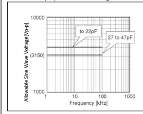
The capacitors less than 22pF can be applied maximum 4.0kV peak to peak at 100kHz or less only for the ballast or the resonance usage in the CFL inverter circuit.
