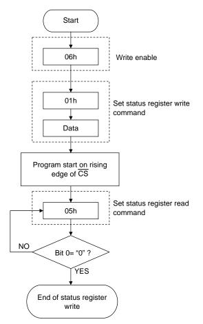
\* Automatically placed in write disabled state at the end of the status register write
