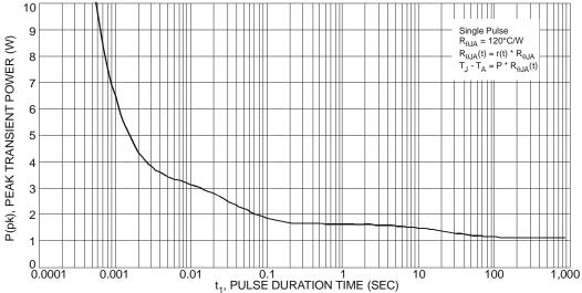
Fig. 1 Single Pulse Maximum Power Dissipation
