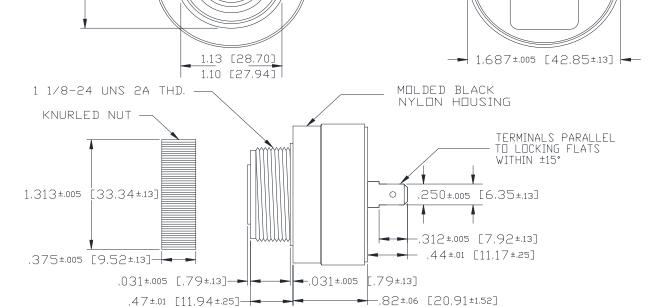
MOUNTING: REMOVE BLACK PLASTIC NUT AND INSERT THREADED FRONT THROUGH 1.25" HOLE PUNCHED IN PANEL, IF ORIENTATION IS NEEDED, NOTE LOCKING FLATS ON DRAWING. SCREW NUT BACK ON. DO NOT OVERTIGHTEN.
