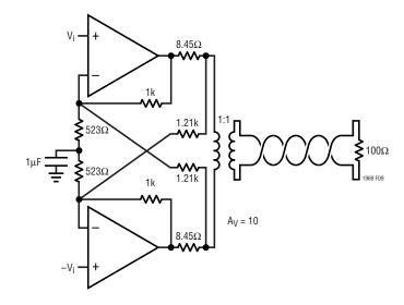
Figure 9. Power Saving ADSL Modem Driver
