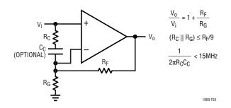
Figure 3. Compensation for Noninverting Gains
