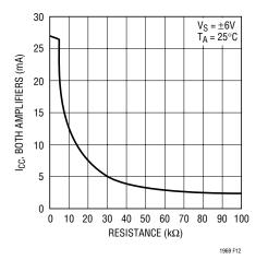
Figure 12. Supply Current vs Control Resistance (R1//R2)
