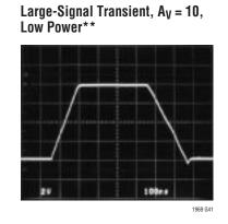
\*13k RESISTOR FROM CTRL1 TO V<sup>-</sup> AND A 49.9k RESISTOR FROM CTRL2 TO V<sup>-</sup> \*\* 49.9k RESISTOR FROM CTRL2 TO V<sup>-</sup>, CTR1 FLOATING
