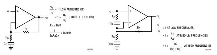
Figure 4. Alternate Noninverting Compensation
