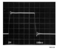
Small-Signal Transient,  $A_V = 10$ ,  $C_L = 1000 pF$ , Low Power\*\*
