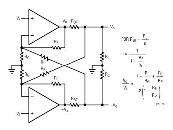
Figure 8. Back-Termination Using Differential Positive Feedback
