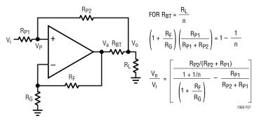
Figure 7. Back-Termination Using Positive Feedback
