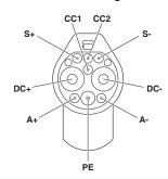
Pin assignment of the Vehicle Connector
