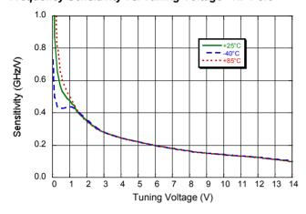
Frequency Sensitivity vs. Tuning Voltage - RF/2 Port
