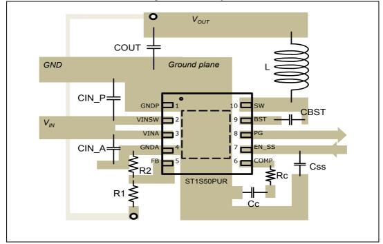
Figure 11. PCB layout
