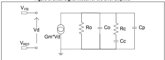
Figure 5. Small signal model for the error amplifier
