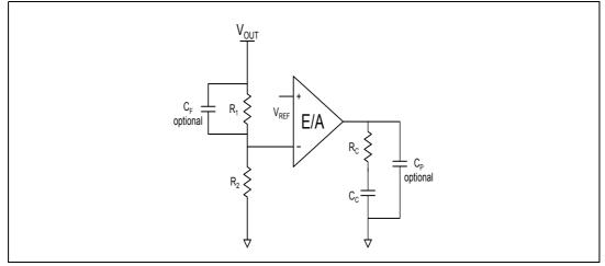
Starting from the target bandwidth ( $f_{BW}$ ) the compensation network values can be calculated to have a stable loop response basing *Equation 22* and *Equation 23*.
