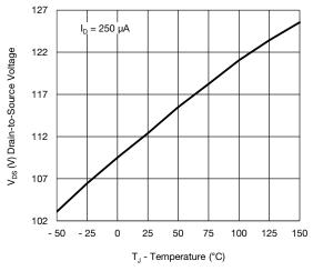
Drain Source Breakdown vs. Junction Temperature
