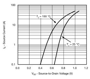
Source-Drain Diode Forward Voltage
