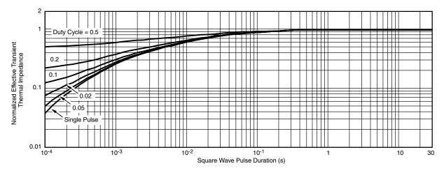
Normalized Thermal Transient Impedance, Junction-to-Case
