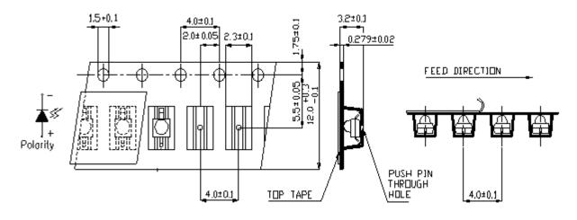
Note: The tolerances unless mentioned are  $\pm 0.1$ , unit=mm.
