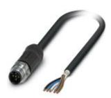
Sensor/Actuator cable, 5-position, PE-X/PE-X halogen-free, black-gray RAL 7021, shielded, Plug straight M12, A-coded, on free cable end, Cable length: 10 m, for outdoor applications, with high-grade steel knurl
