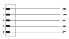
Contact assignment of the M12 plug
