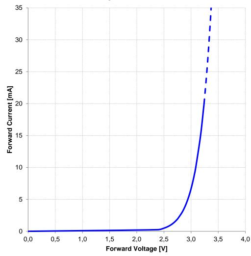
CHECKED GENERAL TOLERANCE PROJECTION METHOD CREATED Würth Elektronik eiSos GmbH & Co. KG EMC & Inductive Solutions PaDi PLD DIN ISO 2768-1m Max-Eyth-Str. 1 74638 Waldenburg **WL-SMCD SMD Mono-color Chip** Tel. +49 (0) 79 42 945 - 0 **LED Diffused** ORDER CODE www.we-online.com 150060BS55040 eiSos@we-online.com DATE (YYYY-MM-DD) BUSINESS UNIT REVISION STATUS PAGE 001.000 Valid 3/7 0603 2017-11-01 **WÜRTH ELEKTRONİK**
