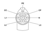
Pin assignment of the Vehicle Connector
