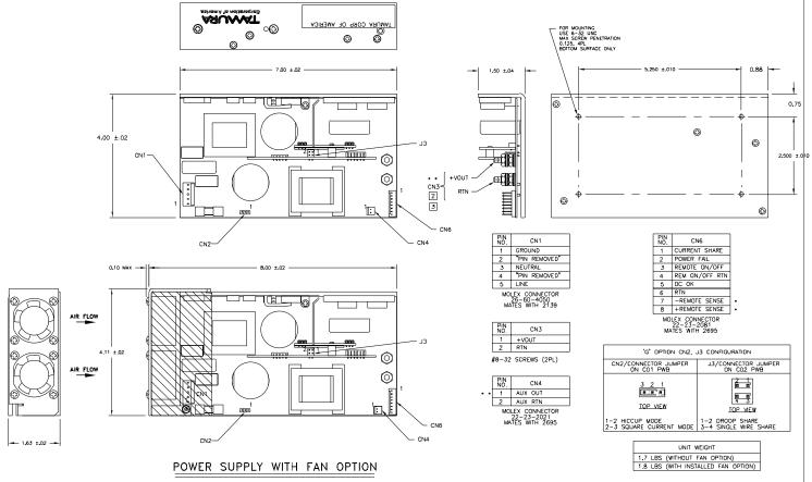
3 OPTIONAL-MOLEX CONNECTOR (OPTION 'K'-LIMITED TO 7A) MAY BE SPECIFIED FOR CN3 INSTEAD OF STANDARD OUTPUT STUDS.
