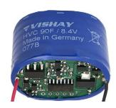
This version is optimized for a 196 HVC in a 90 F, 8.4 V configuration. Basically, it is a voltage converter and switch logic in one, which adjusts to a wide input voltage range. It provides the correct charging voltage and protects against deep discharge.
