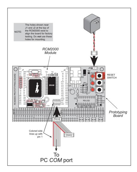
Figure 4. RCM2000 Power and Programming Connections
