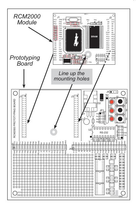
Figure 3. Attaching RCM2000 to Prototyping Board
