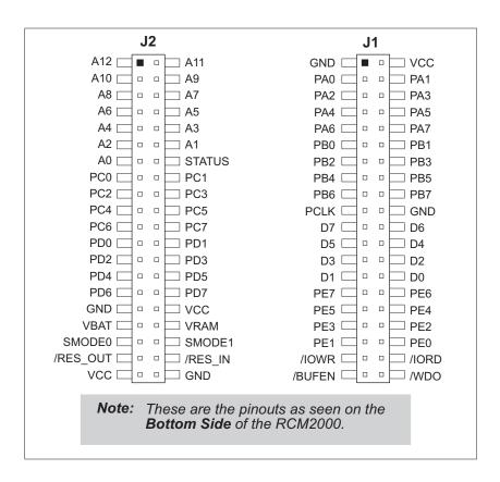
Figure 1. RCM2000 Connector Pinout
