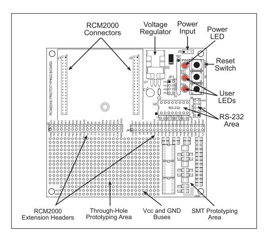
Figure 2. RCM2000 Prototyping Board
