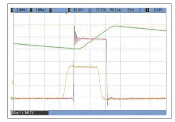
Figure 4: Typical Waveforms for V<sub>IN</sub> = 48 V to 5 V/5 A (1000kHz) Buck converter CH1: VPWM Input voltage — CH2: (IOUT) Switch node current — CH4: (VOUT) Switch node voltage
