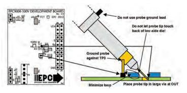
Figure 3: Proper Measurement of Switch Node – OUT
