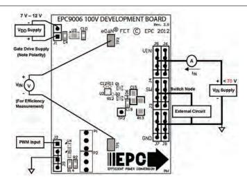
Figure 2: Proper Connection and Measurement Setup
