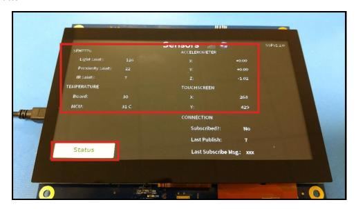
Once the SYG-70CP-DK has successfully connected to the network, the icon representing signal strength will turn green and the **Device ID** will appear. This is the Device ID that will be used to connect to the IBM Watson Quickstart page.
