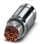
Coupling connector, straight long, shielded: yes, Screw locking, M23, Number of positions: 4+4+4+PE / 3+N +PE, Type of contact: Pin, Crimp connection, Cable diameter: 9 mm ... 12 mm
