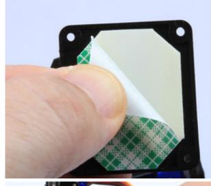
Cut a piece of foam tape to fit in the recess in the bottom of the pan/tilt base. (If you are using narrower tape, you can use multiple pieces.)
