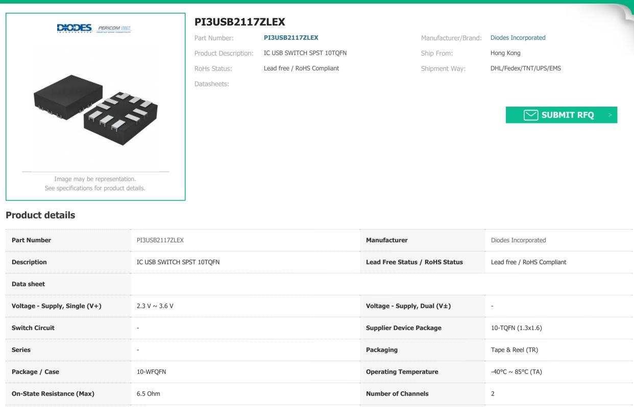
**Multiplexer/Demultiplexer Circuit Moisture Sensitivity Level (MSL)** 1 (Unlimited) 1:1Lead free / RoHS Compliant Lead Free Status / RoHS Status Bi-Directional, USB 2.0 Features **Detailed Description** USB Switch IC 2 Channel 10-TQFN (1.3x1.6) **Base Part Number** PI3USB2117 USB -3db Bandwidth Applications 1.3GHz
